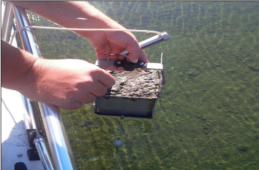
Figure 20. An Ekman hand dredge used to sample sediment macroinvertebrates in Cedar Lake, Van Buren County, Michigan.
