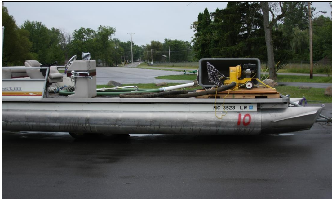
Figure 55. A DASH boat for hand-removal of watermilfoil or other nuisance vegetation. ©Restorative Lake Sciences, LLC
